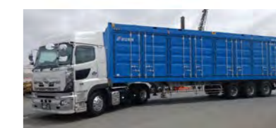
40-foot special container for transport of recyclable resources (HTS has acquired the patent)
