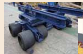
Completed car transport platform (MPB*)
