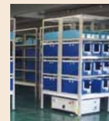
Automated guided vehicle conveys loaded shelves
