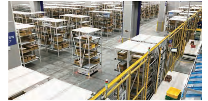
① Picking using a storage shelf conveyance robot "Racrew"
