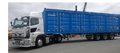
40-foot special container for transport of recyclable resources (HTS has acquired the patent)
