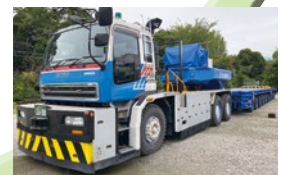
Largest-class trailer in Japan (350 ton capacity)
