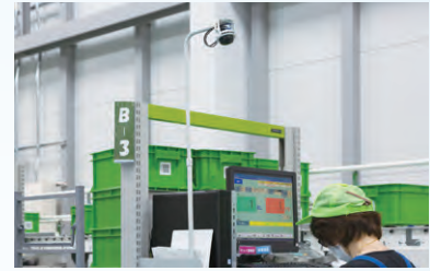
Hand camera used to check work procedures by workers
