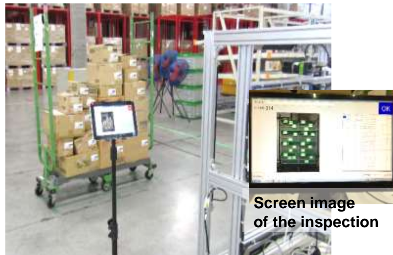
Inspecting barcodes at one-time by image recognition technology
