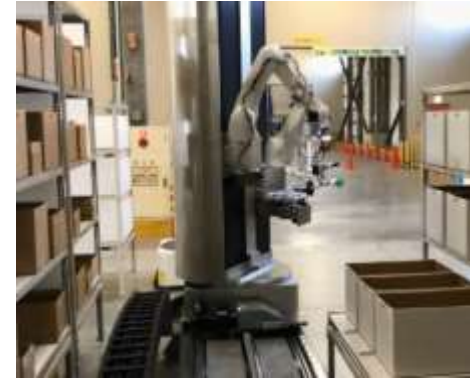
[Ref.] R&D Center: Verifying movable dual-arm piece picking robot
