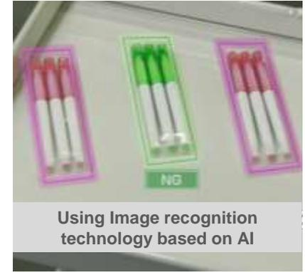
Image recognition inspection system (Preparing to introduction)
