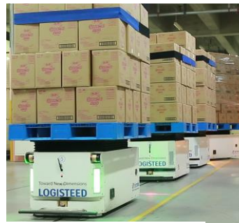
Pallet conveyor AGV
