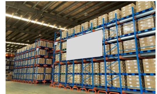
High-density automated horizontal conveyor rack
