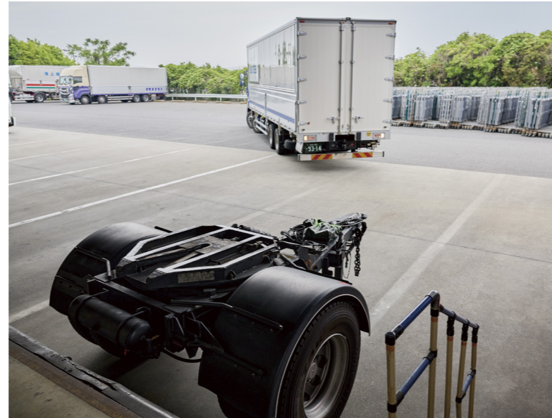
The AEON Kyushu RDC. In front is the coupler, used to connect trailer to trailer. The driver views the built-in camera monitor to back up and connect to the other trailer.
