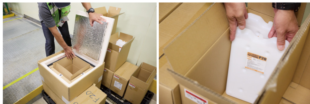
Two photos above: Insulated container used in pharmaceutical transport (left) and heat storage material (right). For instance, where instructions call for storage temperature ranges of 15-25 degrees, heat storage materials that thaw at 20 degrees are utilized.
