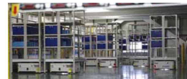
Small/low-floor automated transport vehicle "Racrew" *Racrew is a registered trademark of Hitachi, Ltd. in Japan
