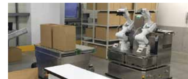
Autonomous dual-arm robot (right) and transport robot (left) work together in a collaborative operations test (picking product from shelves)
